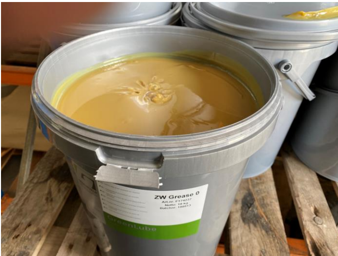
ZW0 Grease - use in any system Grease is thinner than EP2 grease but a similar colour
