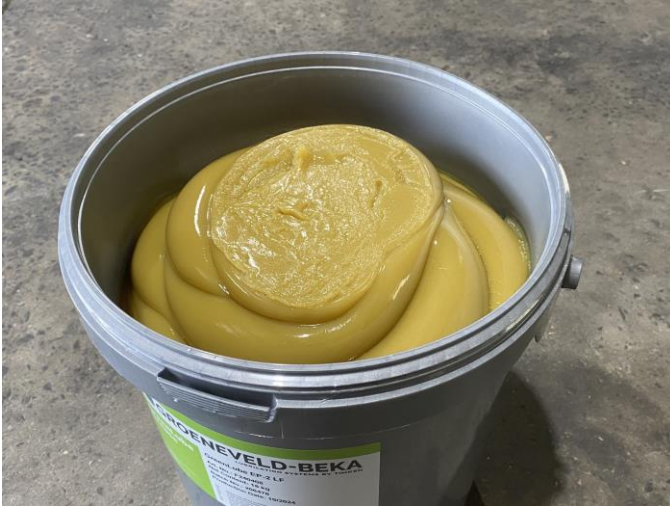
EP2 LF Grease (Lithium Free) - only use in Twin System Grease is quite thick
